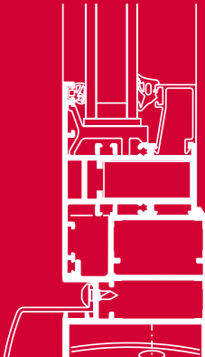
Vertical cross-section of GX frame in FX structure
